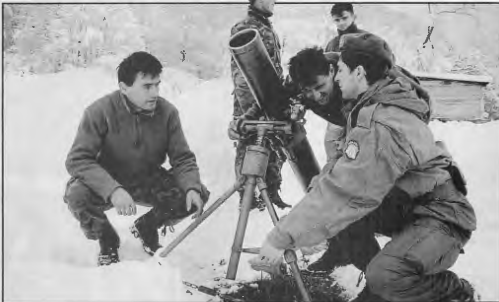
Heavy weapons are in short supply and mortars are a poor man's artillery. MUP troopers train on Yugo M75 120mm mortar, which can handle a full range of ammo, including a rocket-assisted bomb with a range of nearly 10 klicks.
